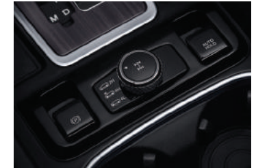
Electronic parking brake with auto-hold function
