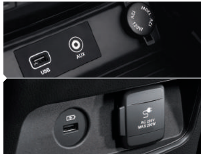
USB port and power outlet on centre console, USB port and 220V/115V inverter in 2 nd row
