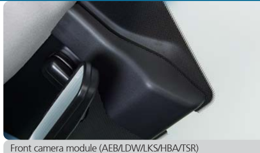
Front camera module (AEB/LDW/LKS/HBA/TSR) with rain sensing and automatic light control unit
