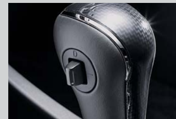
Tip switch manual mode with 6-speed automatic
