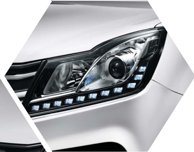
25-watt HID head lamps & LED daylight running lights
