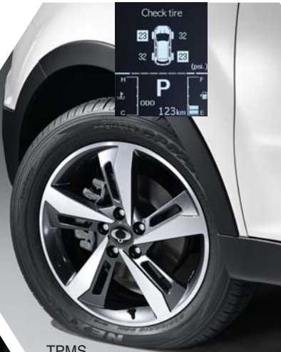
TPMS (Tyre Pressure Monitoring System)
