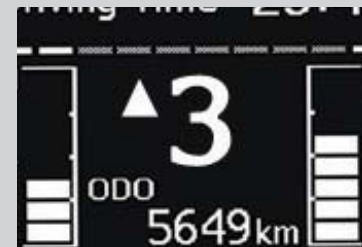
Gear shift indicator with 6-speed manual
