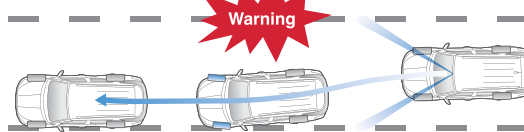
STEP3 System temporarily takes control of steering
