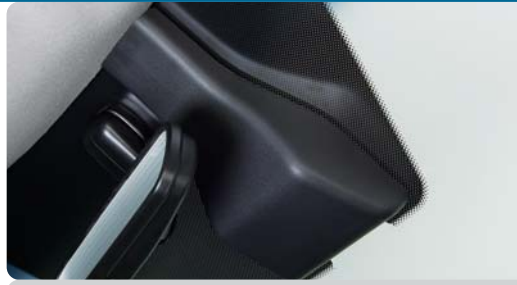
Front camera module (AEB/LDW/LKS/HBA/TSR) with rain sensing and automatic light control unit
