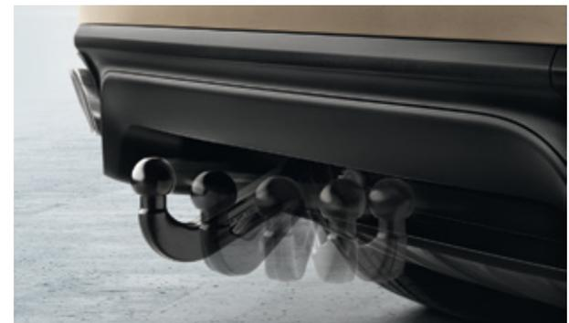
Towbar system with electrically deployable towball
