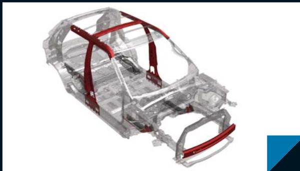
Ultra-high-tensile steel plate at ten key points in the frame to further enhance occupant safety.
