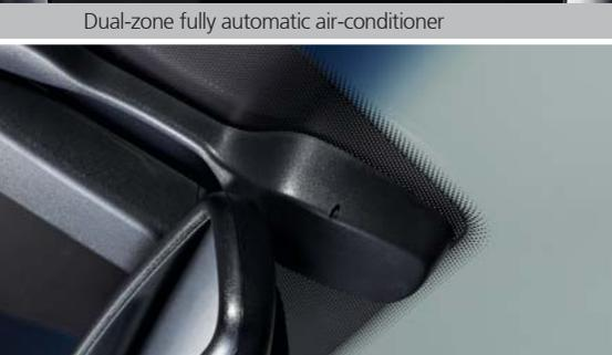
Rain sensing and automatic light control unit
