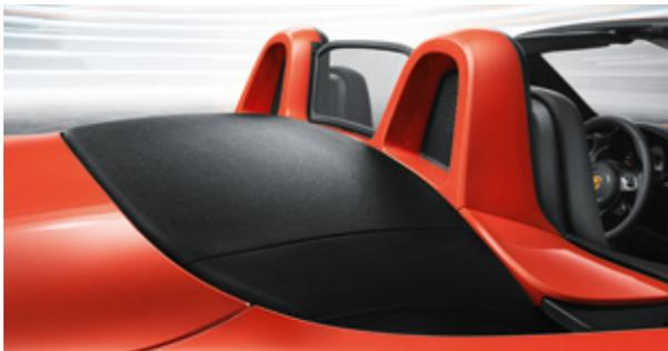
Roll-over bars painted in exterior colour, net-type wind deflector
